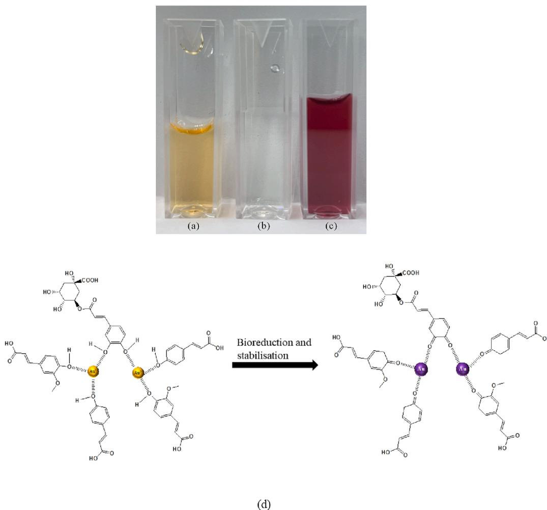
Fig. 2. Image of (a) Peel extract, (b) gold salt solution, (c) Au NPs and (d) proposed formation mechanism of Au NPs.
