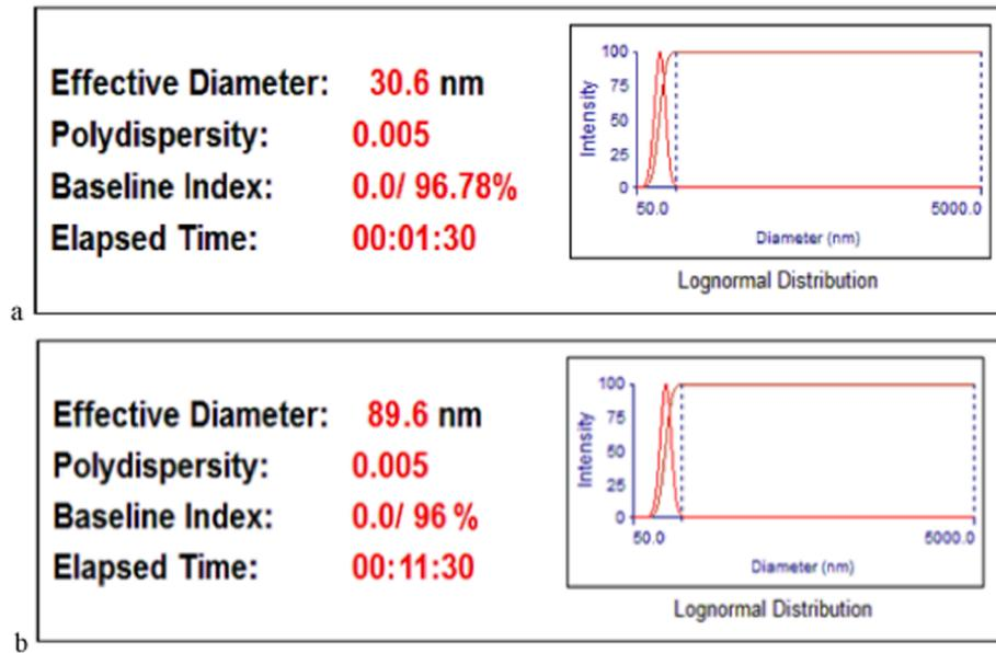
Fig. 4. a) particle size analysis of the calcined binary composite nanopowder at temperatures (650 °C), b) particle size analysis of the calcined binary composite nanopowder at temperatures (750 °C).
