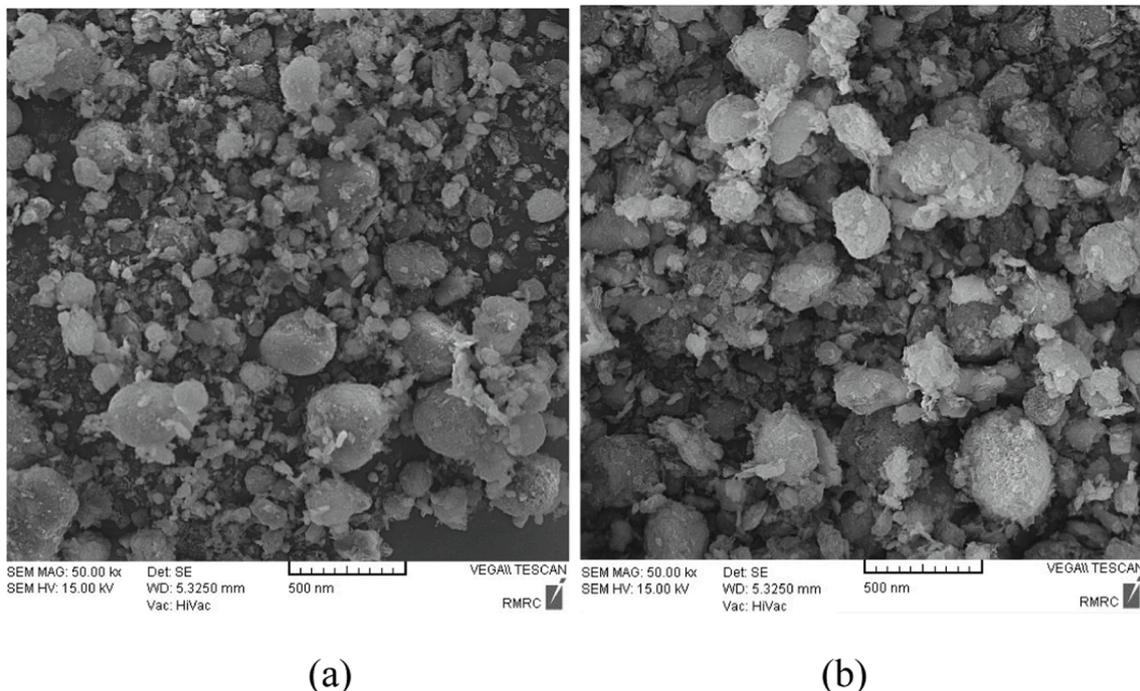
Fig. 5. a) sem of the calcined binary composite nanopowder at (a) 650 °C and (b) 750 °C.
