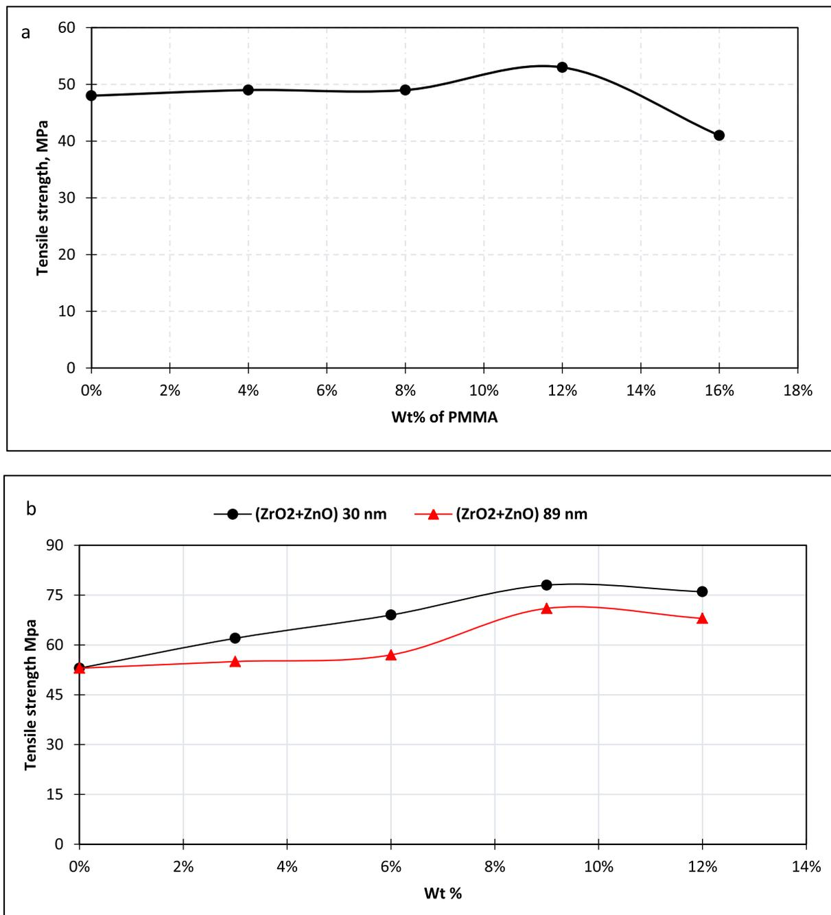
Fig. 6. Maximum tensile strength a) From dding (methyl vinyl silicone resin) to (lamination resin), b) the polymeric blend reinforcement by binary nanocomposite powder.
