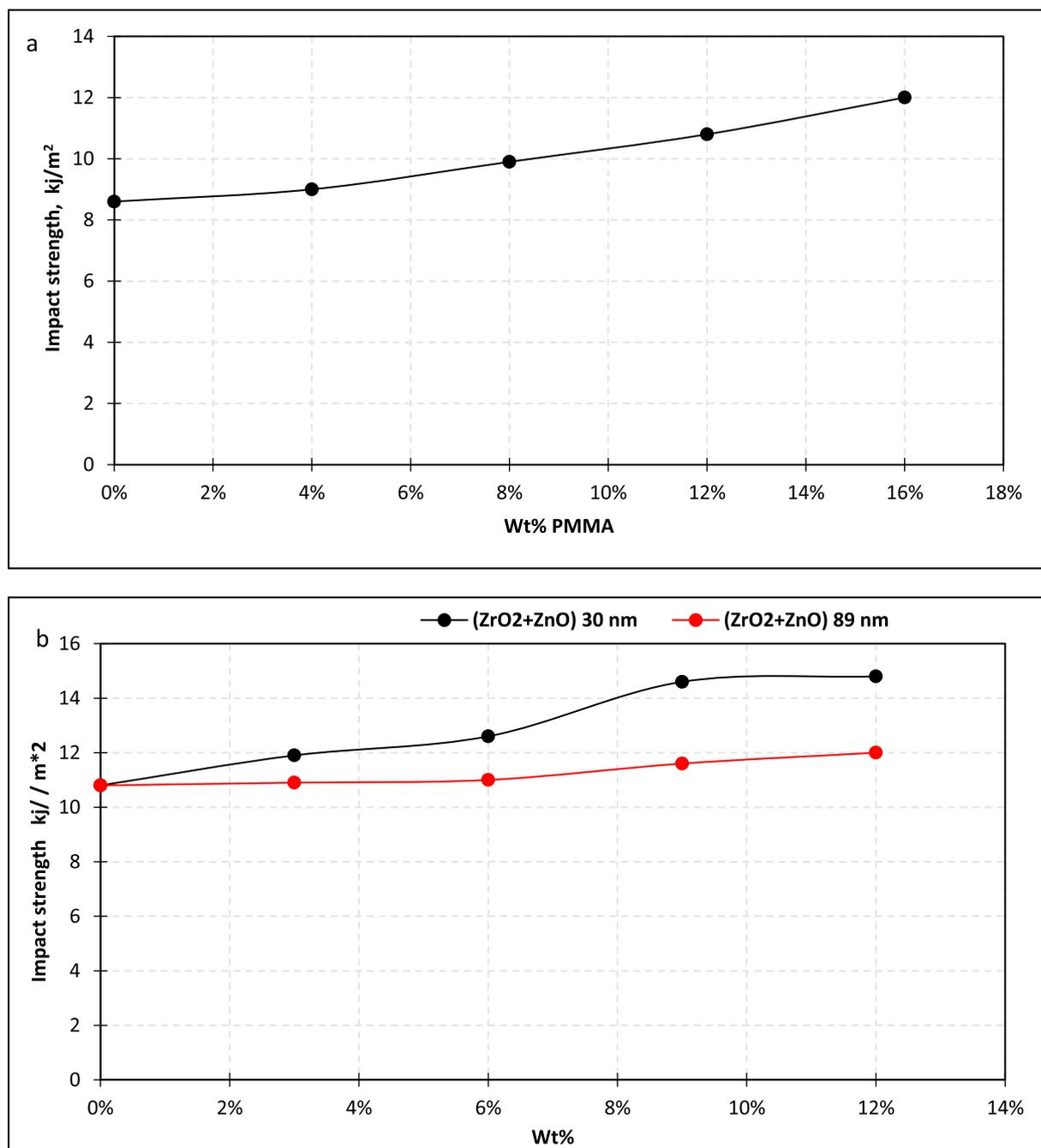
Fig. 8. Impact strength a) From dding (methyl vinyl silicone resin) to (lamination resin), b) the polymeric blend reinforcement by binary nanocomposite powder.
