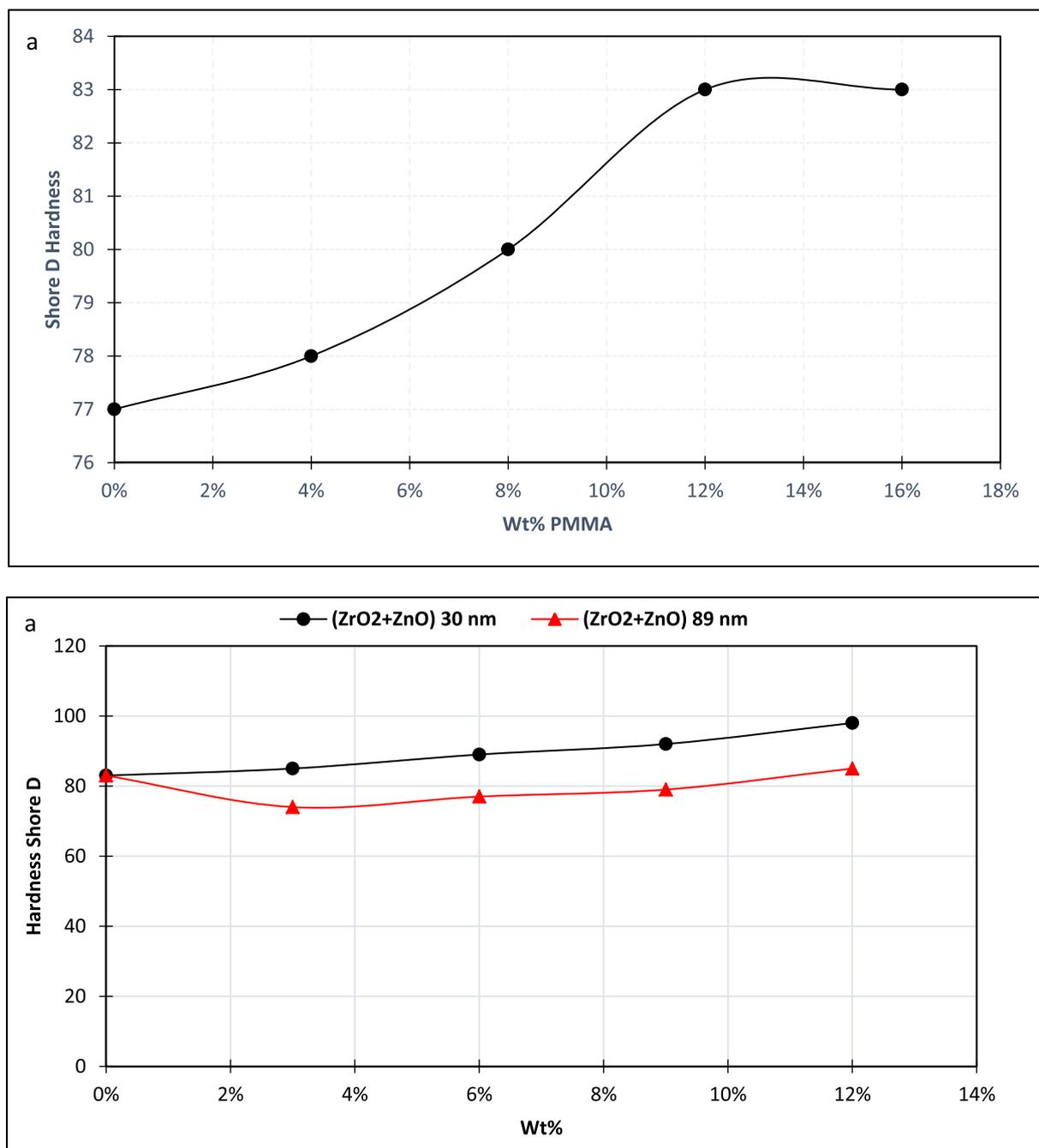
**Fig. 9.** The hardness shore d a) from dding (methyl vinyl silicone resin) to (lamination resin), b) the polymeric blend reinforcement by binary nano-composite powder.
