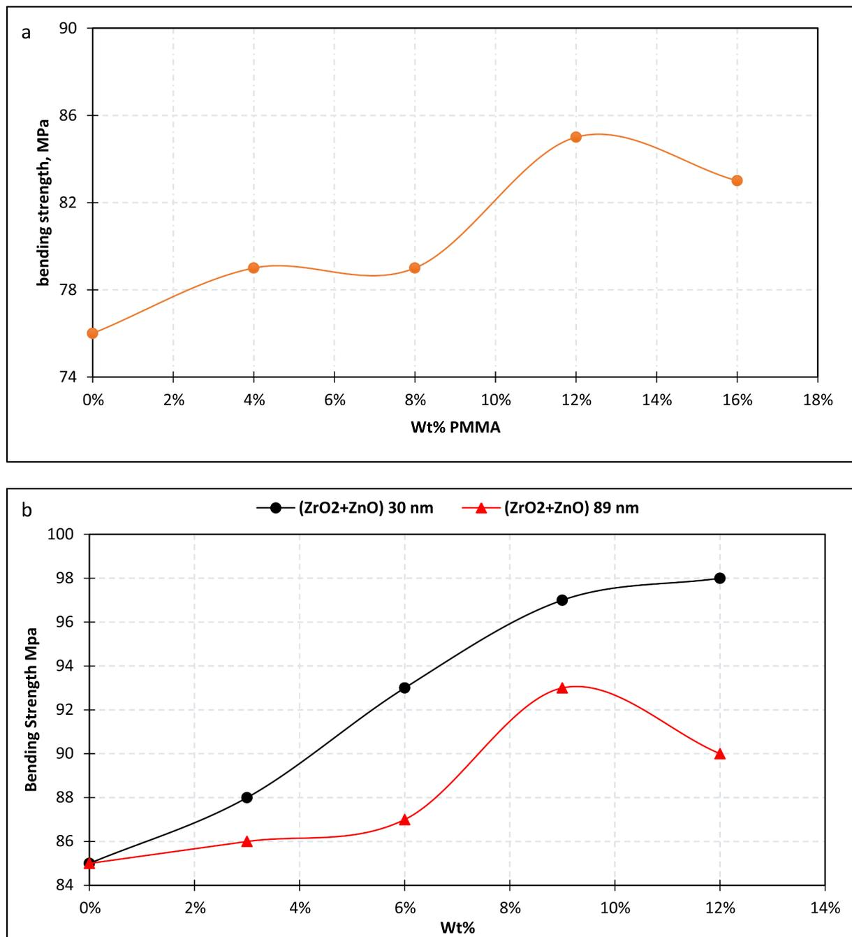
Fig. 7. Maximum bending strength a) From adding (methyl vinyl silicone resin) to (lamination resin), b) the polymeric blend reinforcement by binary nano-composite powder.
