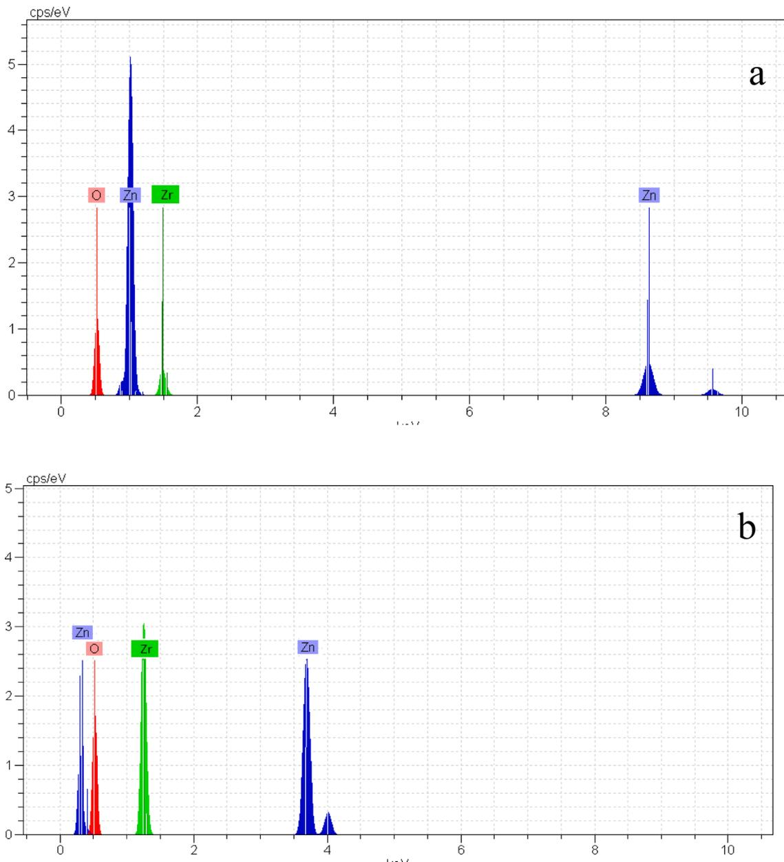
**Fig. 2.** a) the chemical composition of the calcined binary composite nanopowder at temperatures (650 °C); b) the chemical composition of the calcined binary composite nanopowder at temperatures (750 °C).
