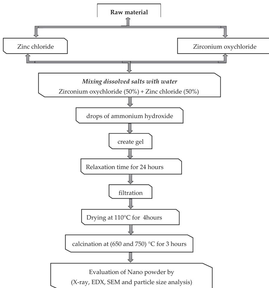
Fig. 1. Flowchart showing the procedure for preparing the binary composite Nanopowders.
