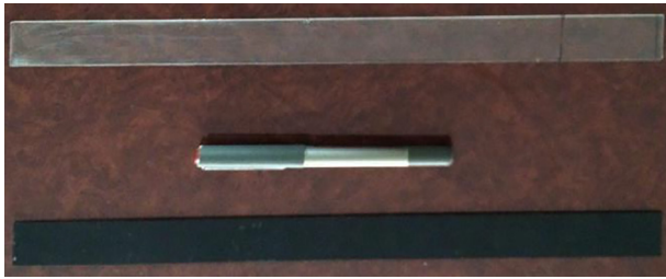
Fig. 10. Typical SWNT-c/epoxy (0.1 wt%) and pure epoxy resin test samples.
