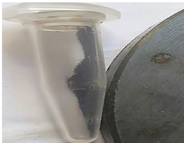
Fig. 2. Demonstration of the attraction potential of Cellulase/Iron oxide magnetic composites (CMNPS) towards a magnet kept aside.
