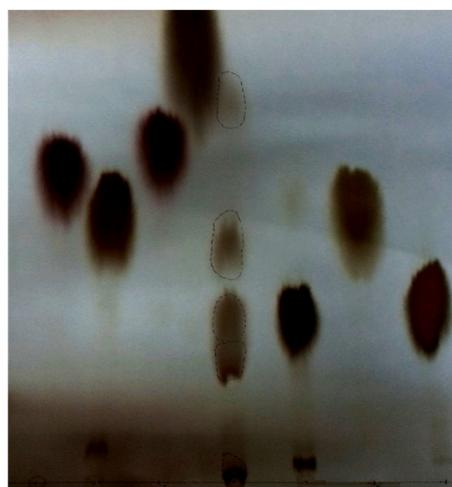
Fig. 2. Paper chromatograph of the hydrolyzed produced EPS.
