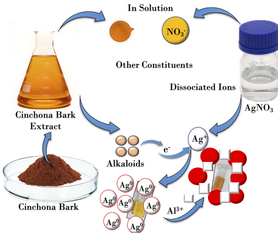
Scheme 1. Schematic representation of the synthesis of C-AgNPs and their aggregation in the presence of Al 3+ .
