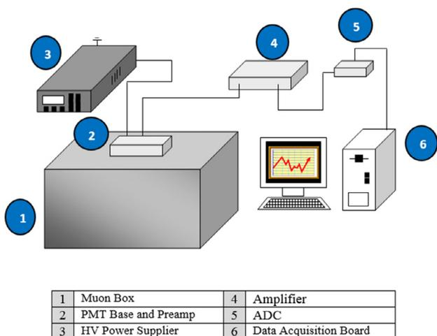
Fig. 1. Schematic diagram showing the main components of the KACST 1 m<sup>2</sup> CR scintillator-based detector.
