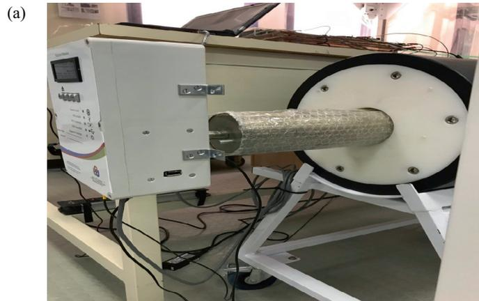
Fig. 5a. photograph shows the mini neutron monitor installed at the KACST station.
