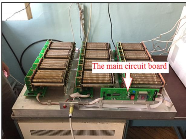
Fig. 6. view of the CARPET detection unit.
