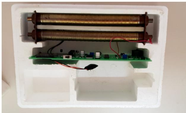
Fig. 8. Single charged particle detector based on two Geiger counters.
