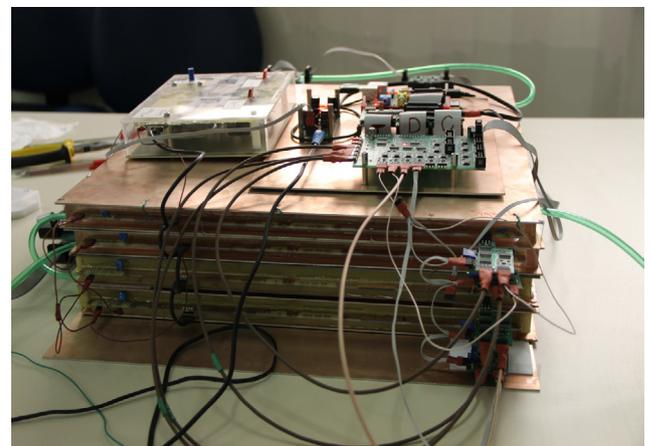
**Fig. 3.** Photograph shows the KACST developed 40 × 40 cm<sup>2</sup> MWPC.
