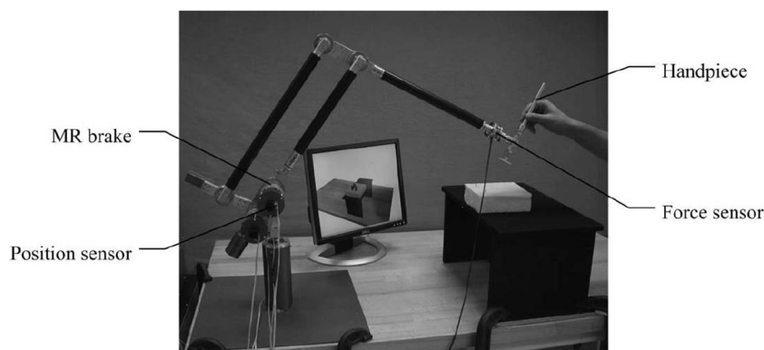
Fig. 9. A haptic interface with MR brake for dental implant surgery (Senkal et al., 2011).
