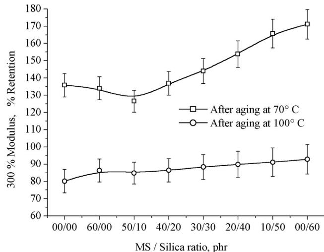
**Figure 3** Percentage retention V/S marble sludge/silica loading on 300% modulus of hybrid natural rubber composites.
