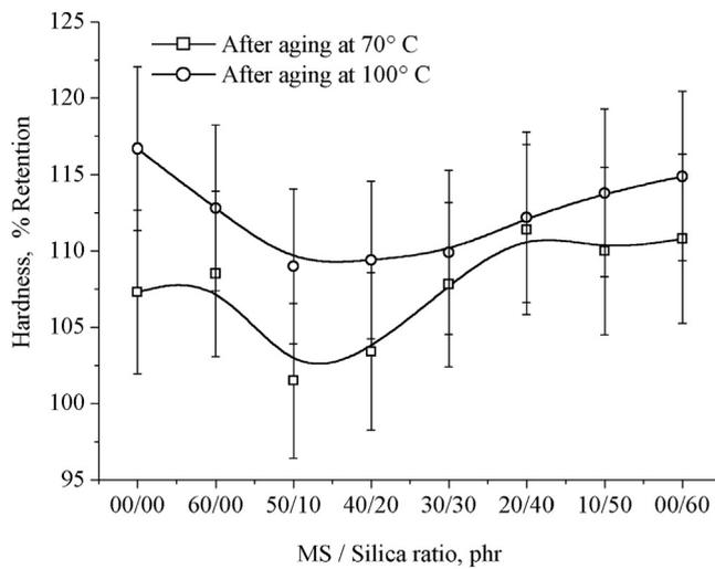
**Figure 6** Percentage retention V/S marble sludge/silica loading on hardness of hybrid natural rubber composites.
