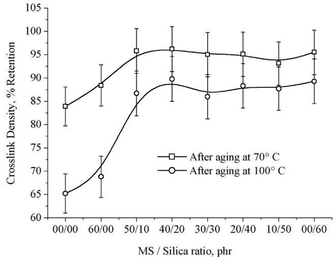
**Figure 8** Percentage retention V/S marble sludge/silica loading on crosslink density of hybrid natural rubber composites.
