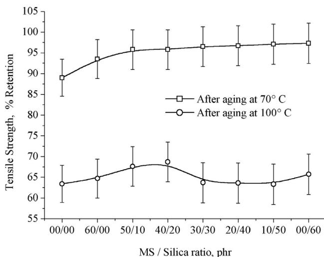
**Figure 1** Percentage retention V/S marble sludge/silica loading on tensile strength of hybrid natural rubber composites.
