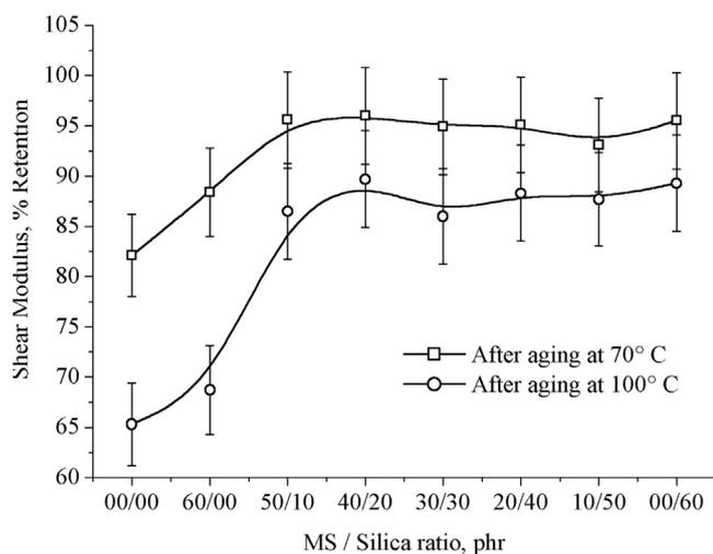
**Figure 9** Percentage retention V/S marble sludge/silica loading on shear modulus of hybrid natural rubber composites.
