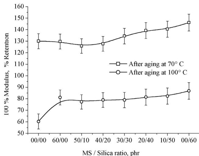
**Figure 2** Percentage retention V/S marble sludge/silica loading on 100% modulus of hybrid natural rubber composites.
