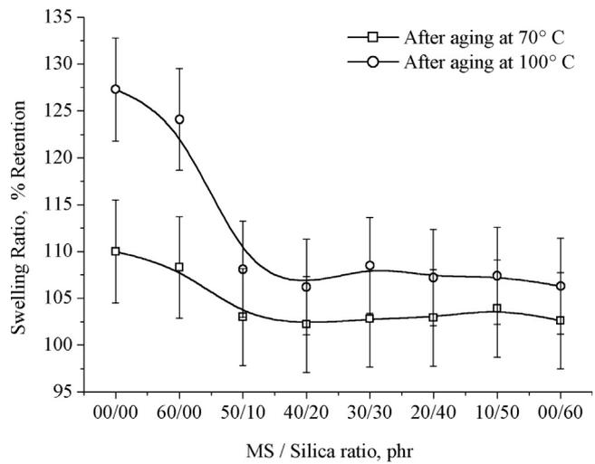
**Figure 7** Percentage retention V/S marble sludge/silica loading on swelling ratio of hybrid natural rubber composites.
