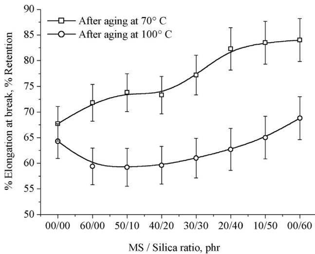
**Figure 5** Percentage retention V/S marble sludge/silica loading on % elongation at break of hybrid natural rubber composites.
