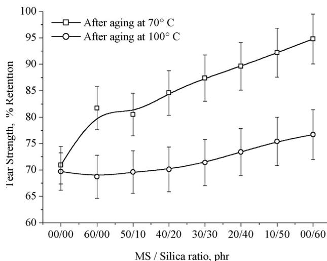
**Figure 4** Percentage retention V/S marble sludge/silica loading on tear strength of hybrid natural rubber composites.
