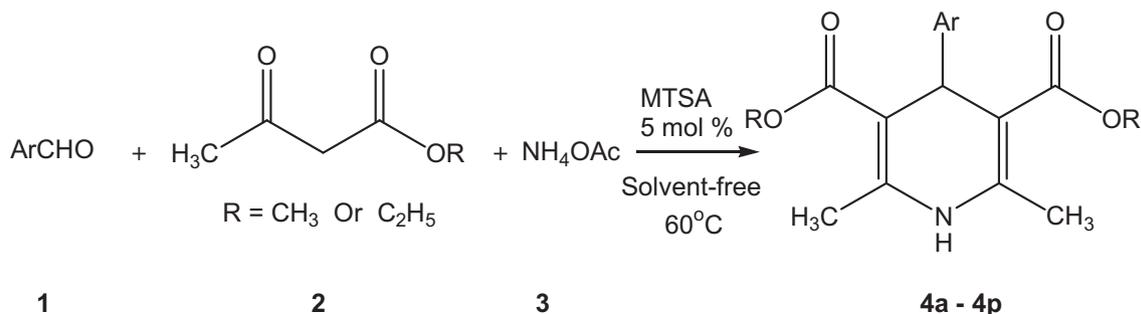
**Scheme 2** The reaction of aromatic aldehyde, ethyl/methyl acetoacetate and ammonium acetate in the presence of MTSA as catalyst at 60 °C under solvent free condition.
