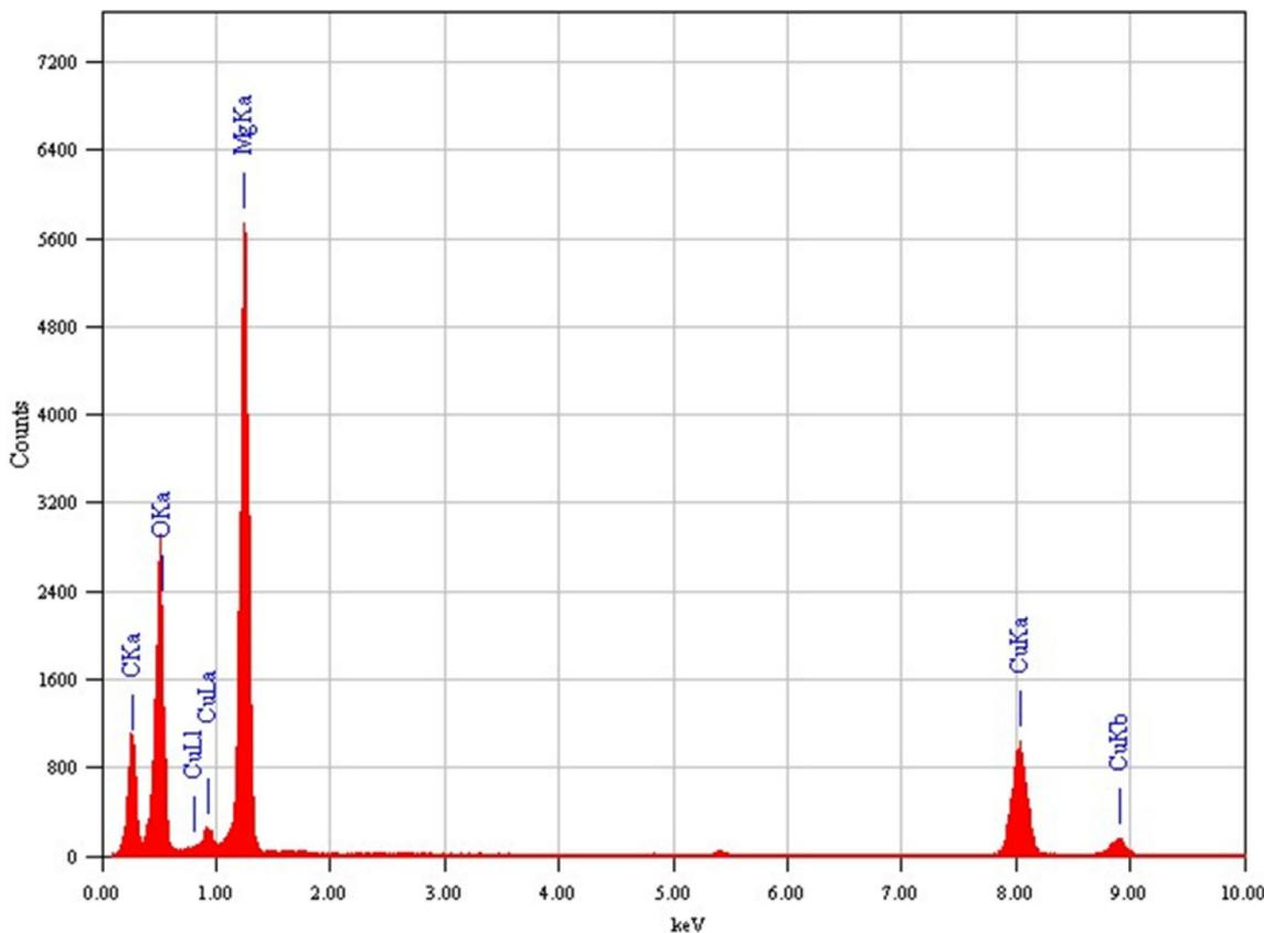
Fig. 4. TEM-EDX spectra of MgO nanoparticles.
