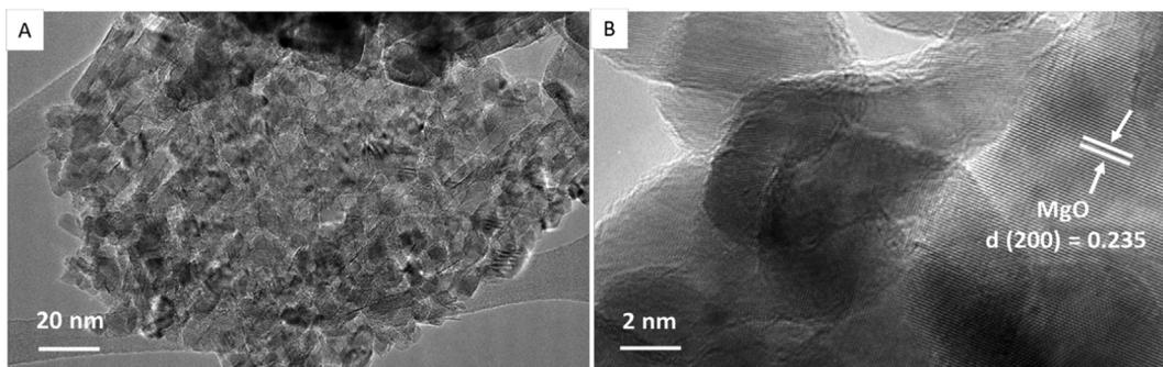
Fig. 3. Low-resolution (A) and high-resolution (B) FETEM micrographs of MgO nanoparticles.
