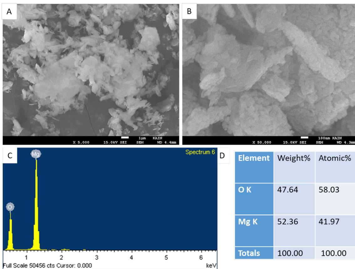
Fig. 2. FESEM micrographs of MgO nanoparticles of different magnifications (A and B). SEM-EDX spectra (C) and elemental composition (D) of MgO nanoparticles.
