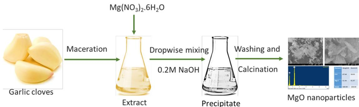
Fig. 1. Illustration of green process MgO nanoparticles synthesis using garlic extract.
