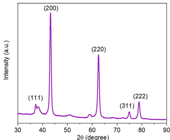
Fig. 5. XRD pattern of MgO nanoparticles.
