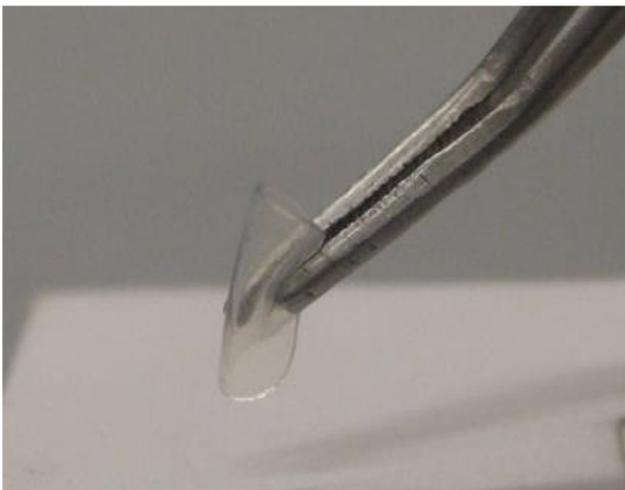
Fig. 9. Picture of manually folded Ss-PS lens.
