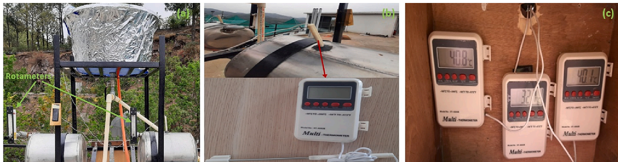
Fig. 2. (a) Rotameters (b) Digital thermometer (c) Display units.
