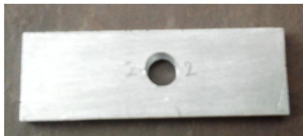
**Fig. 1.** Specimen for slurry erosion tester.
