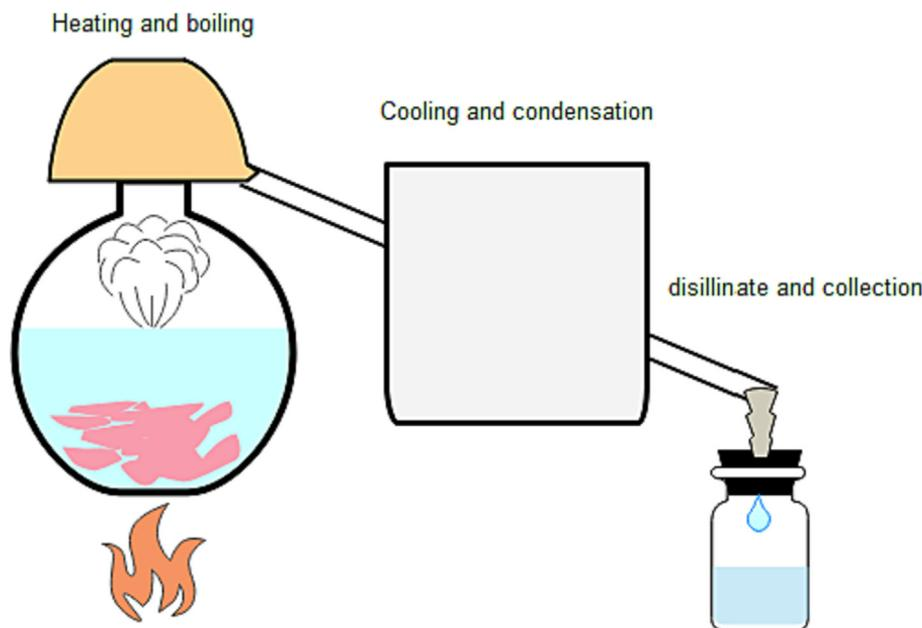
Fig. 1. Schematic view of Taif rose traditional distillation technology.
