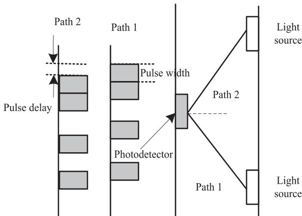
Fig. 1. Inter-symbol interference due to multi-path transmission delay.
