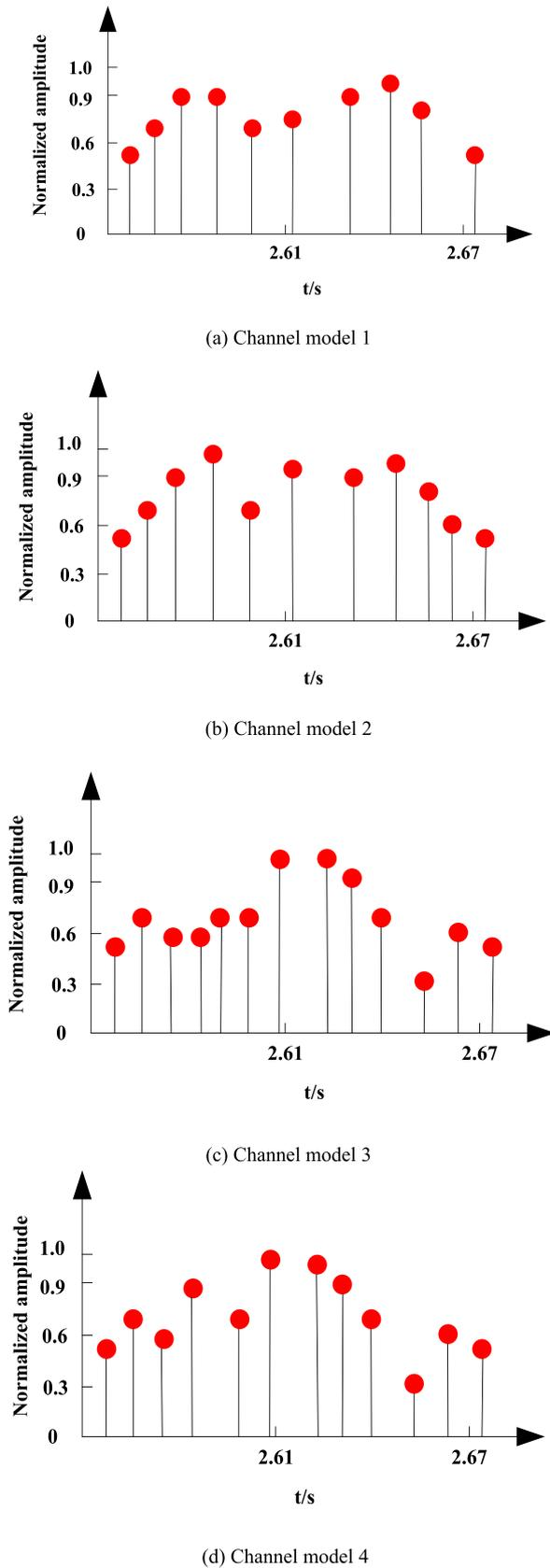
Fig. 8. Channel impulse response output of communication system.
