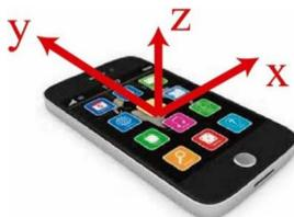
**Fig. 4.** Orientation of the axis in a Smartphone. The measurements are made in the direction of the 'y' axis which must be perpendicular to the North-South axis.
