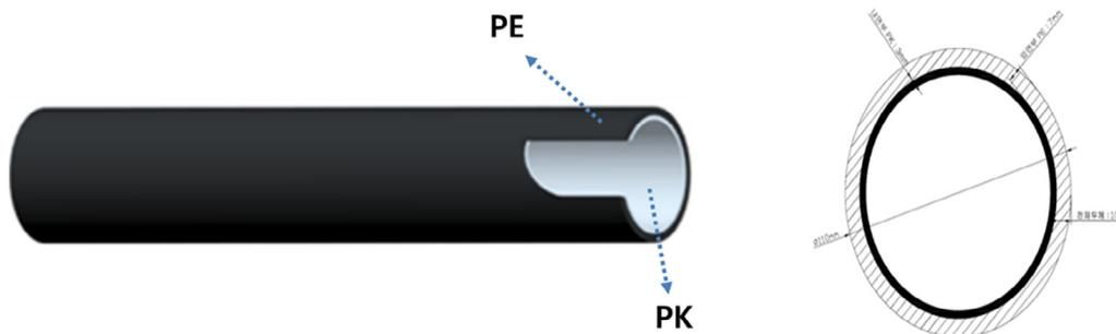
Fig. 1. Details of PE and PK double layer pipe.
