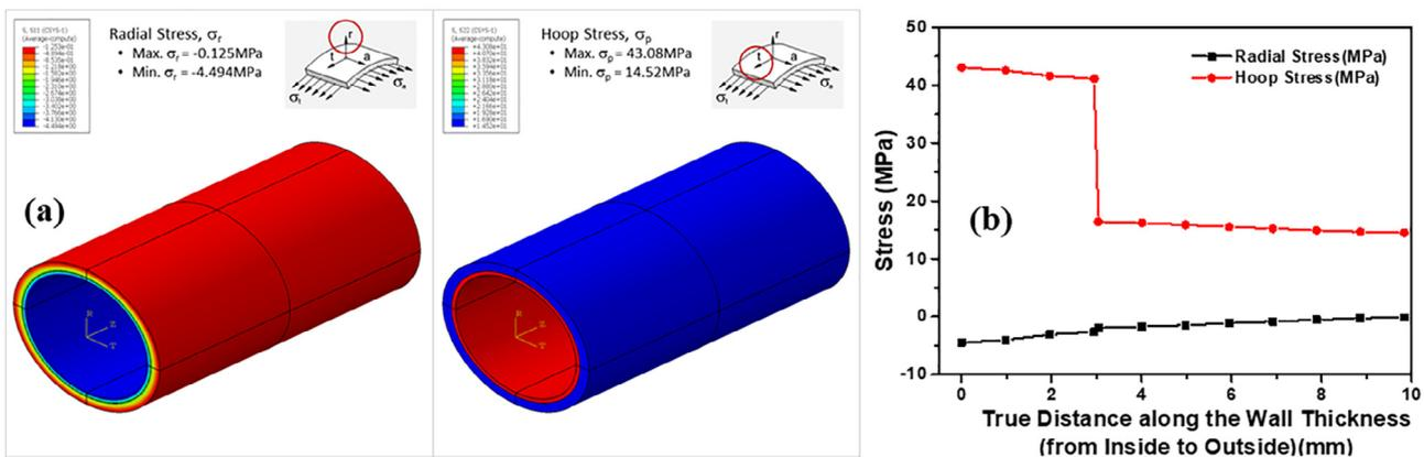
Fig. 4. Radial stress and hoop stress analysis of the PE and PK double layer pipe at internal pressure condition of 5.0 MPa.
