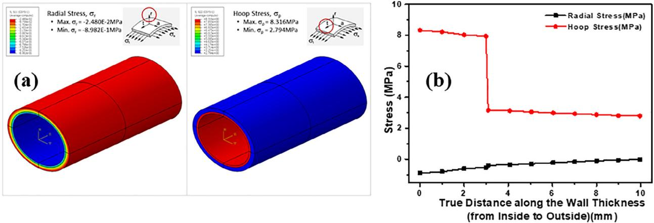
Fig. 2. Radial stress and hoop stress analysis of the PE and PK double layer pipe at internal pressure condition of 1.0 MPa.
