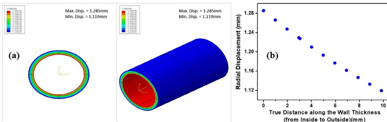
Fig. 5. Radial displacement of the PE and PK double layer pipe at internal pressure condition of 5.0 MPa.
