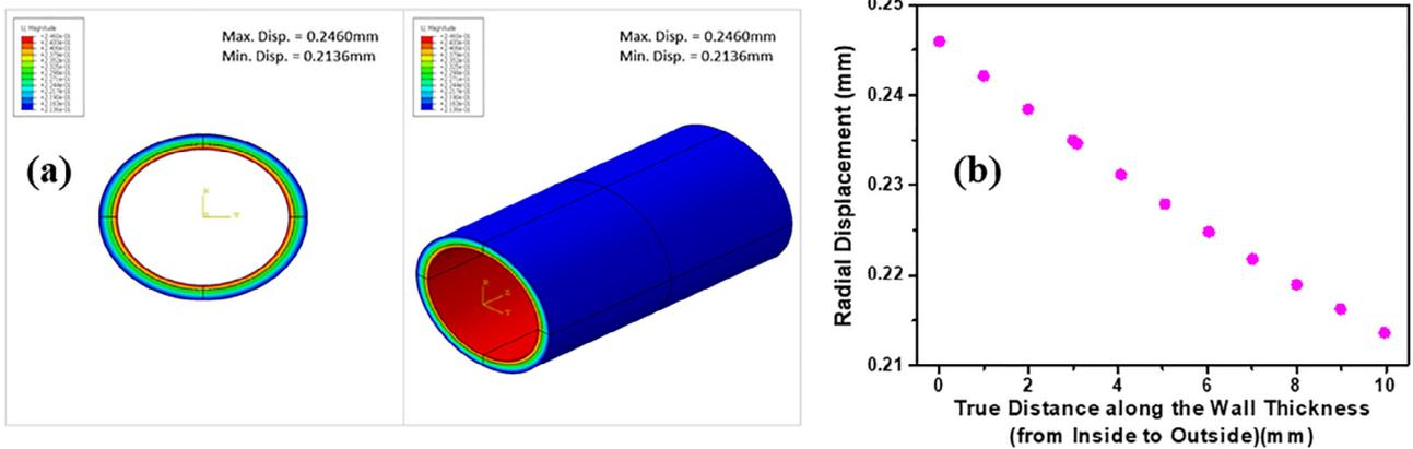
Fig. 3. Radial displacement of the PE and PK double layer pipe at internal pressure condition of 1.0 MPa.
