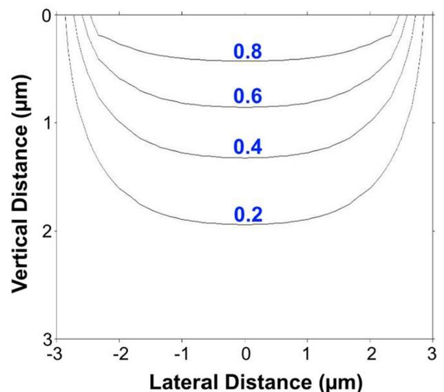
Fig. 5. Displays the calculation by FDM in IONEX for Silver ion concentration distribution.
