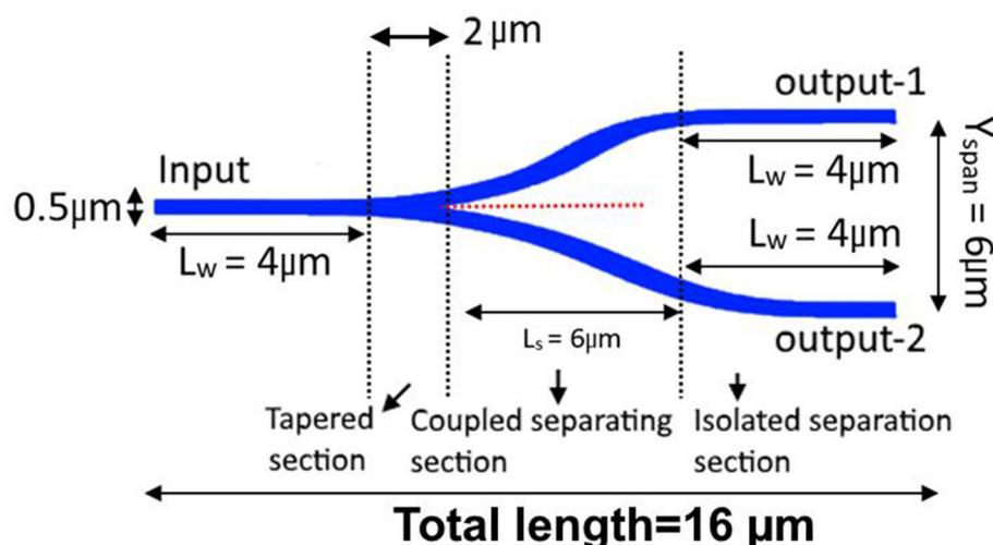
**Fig. 6.** Illustrates the three different sections of the splitter design according to the parameters presented in Table 2.
