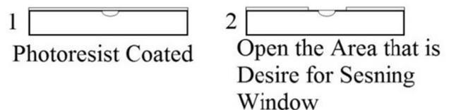
**Fig. 2.** The processing configurations for producing the sensor, (1). Coat the photoresist with a spin coater (2). Open the window by using mask and UV exposure with considering of developer.
