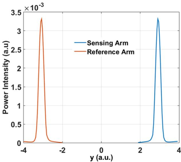
Fig. 8. Optical power output without DNA implementation.
