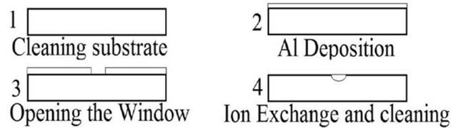
**Fig. 1.** Shows the processing configurations for ion-exchange, (1). Clean the glass substrate precisely (2). Al deposition with using the sputtering machine (3) using photoresist and within the usage of UV open the window that we want to open the channel and wet etching (4). Ion-exchange with using 400 °C in the molten salt after that clean the substrate precisely.
