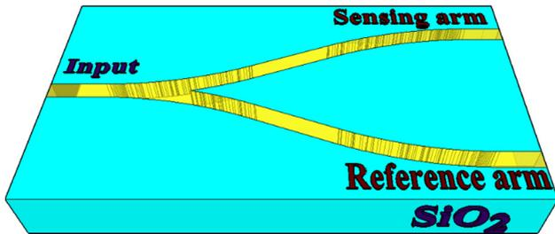
Fig. 4. The different regions structure of splitter waveguide.
