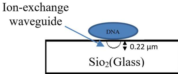
Fig. 3. Showing the DNA on top of the ion-exchange waveguide in case of sensing.
