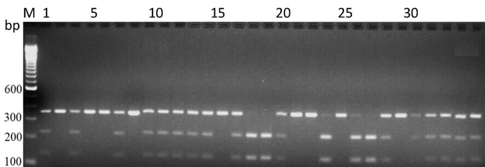
**Fig. 2.** RFLP analysis for the single nucleotide polymorphism of *ITGB3* gene (T1565C) mutation on PCR fragments cutting with *NciI* respectively (Table 2).
