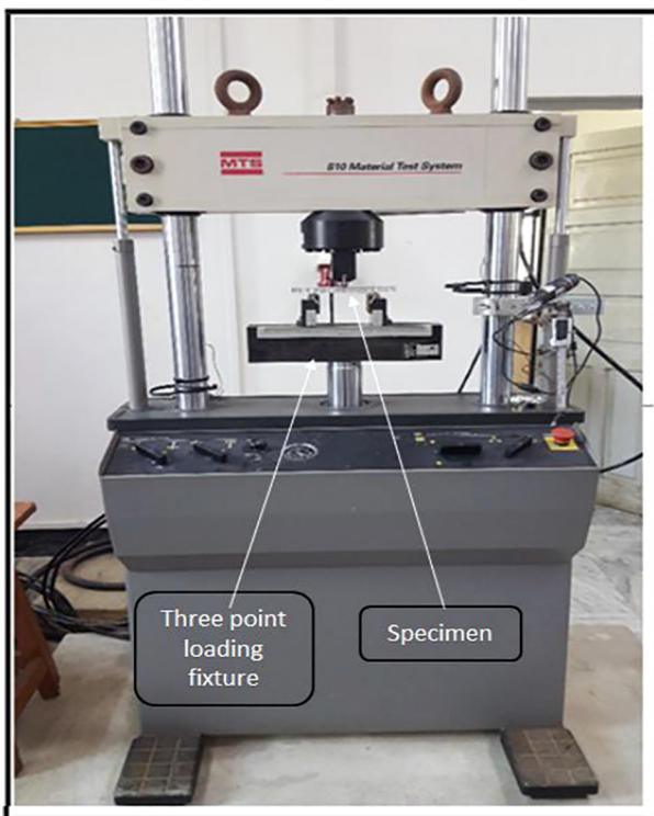
Fig. 2. Experimental setup and three point loading arrangement.
