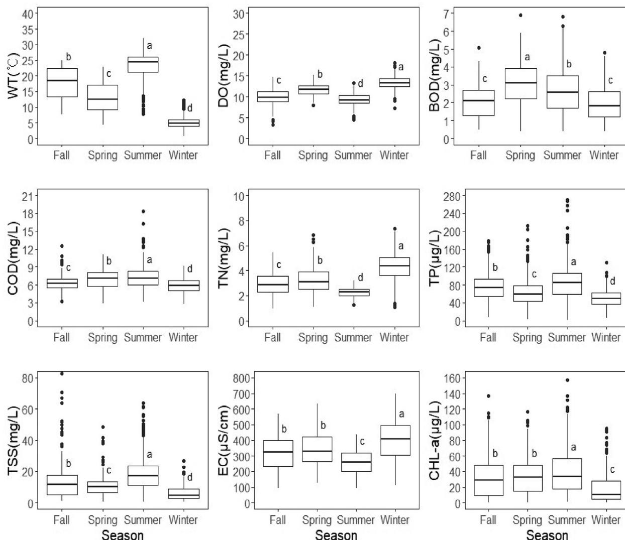
Fig. 3. Variation in water temperature (WT), dissolved oxygen (DO), nutrients (TP: total phosphorus, TN: total nitrogen), organic matters (BOD: biological oxygen demand, COD: chemical oxygen demand), suspended solids (TSS: total suspended solids), electrical conductivity (EC) and algal chlorophyll (CHL-a: chlorophyll-a) based on the season (Spring: Mar-May, Summer: Jun-Aug, Fall: Sep-Nov, Winter: Dec-Feb) in the Geum River.
