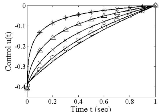
Fig. 4. Optimal control  $u(t)$  for different  $\alpha$  for the fixed final time-free final state problem (\* :  $\alpha = 0.45$ ,  $\Delta$  :  $\alpha = 0.6$ ,  $\times$  :  $\alpha = 0.75$ ,  $O$  :  $\alpha = 0.9$ , – :  $\alpha = 1.0$ ).
