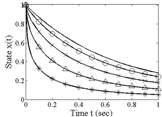
Fig. 3. Optimal state  $x(t)$  for different  $\alpha$  for the fixed final time-free final state problem (\* :  $\alpha = 0.45$ ,  $\Delta$  :  $\alpha = 0.6$ ,  $\times$  :  $\alpha = 0.75$ ,  $O$  :  $\alpha = 0.9$ , – :  $\alpha = 1.0$ ).
