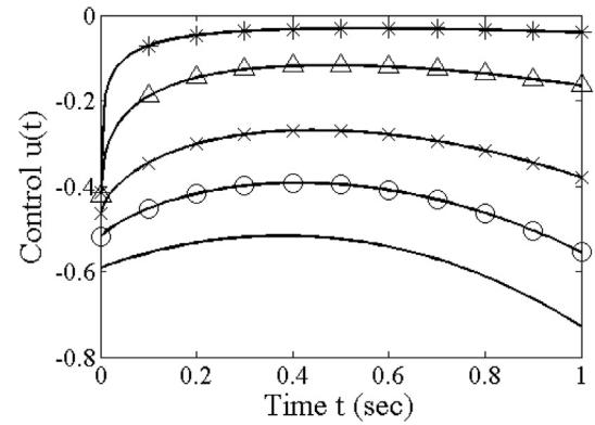
Fig. 2. Optimal control  $u(t)$  for different  $\alpha$  for the fixed final time-fixed final state problem (\* :  $\alpha = 0.35$ ,  $\Delta$  :  $\alpha = 0.5$ ,  $\times$  :  $\alpha = 0.7$ ,  $O$  :  $\alpha = 0.85$ , – :  $\alpha = 1.0$ ).
