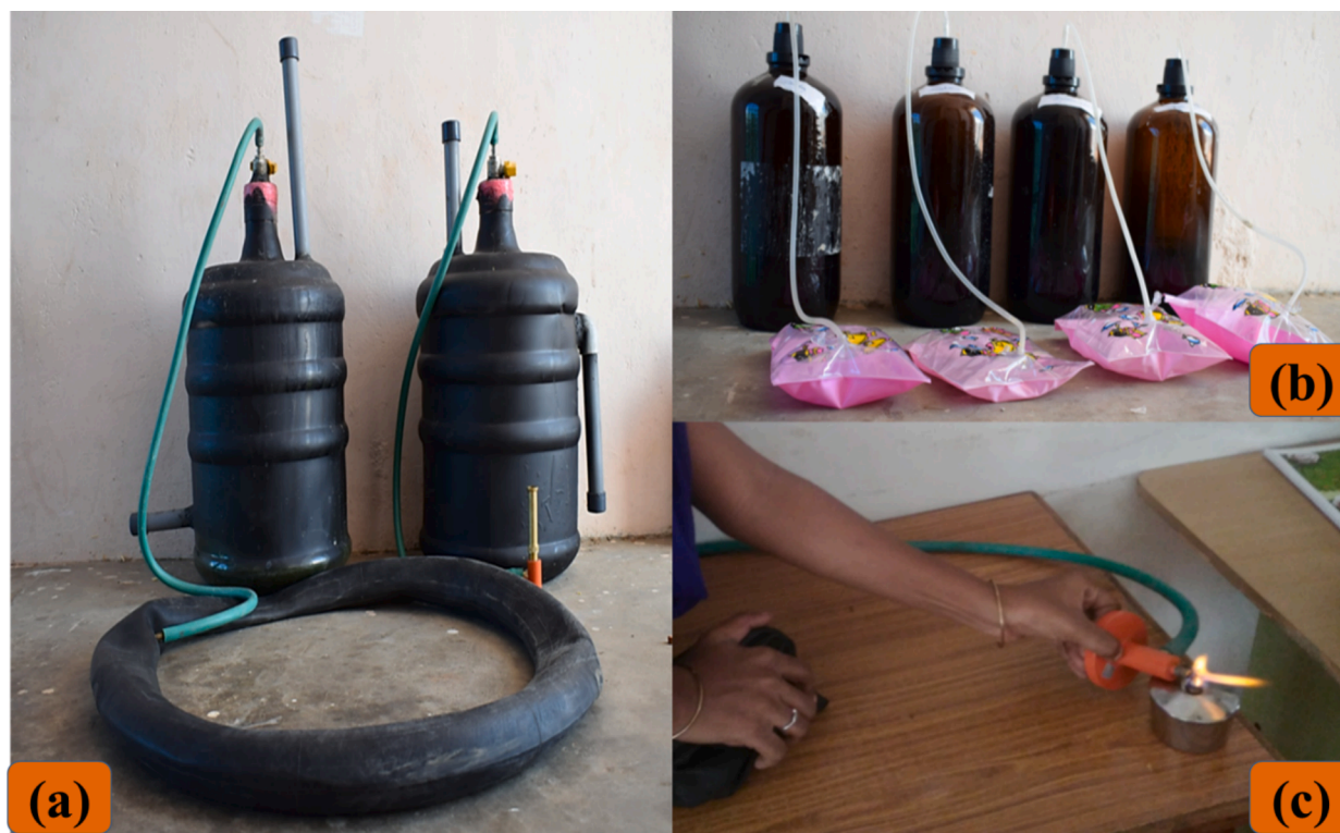
Fig. 2. (a) Anaerobic laboratory digesters; (b) Gas collecting methods (c) Flame experiment.
