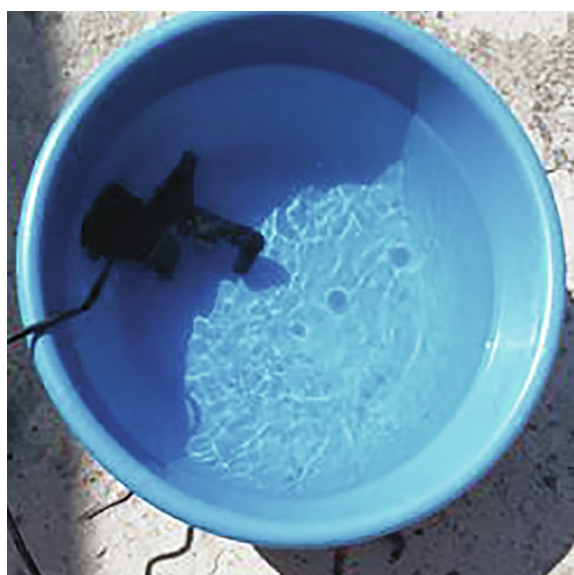
Fig. 3. A comparative evaporation reduction method in which water was recirculated by means of a pump.
