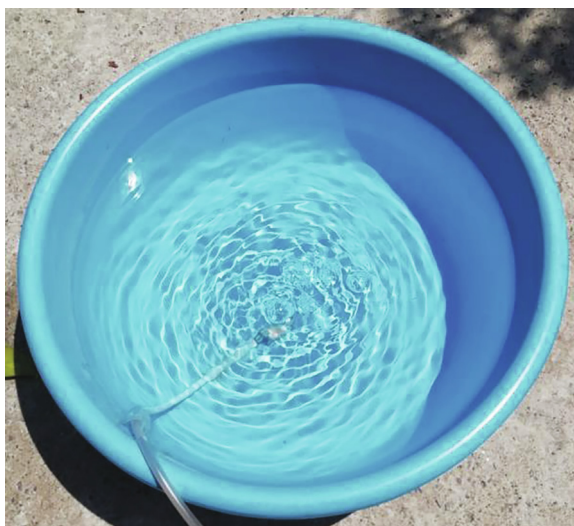
Fig. 2. A comparative evaporation reduction method in which an air pump and hose introduced an air bubble plume in the center of the bottom surface of the container.
