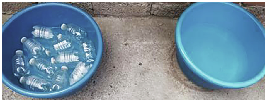
Fig. 1. The control container (on the right, no evaporation reduction method) and the container with the evaporation reducer currently under study (on the left, with PET bottles to cover the water surface).
