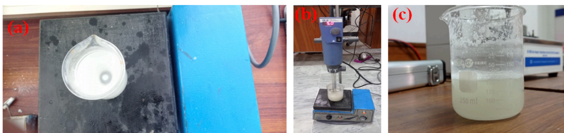
Fig. 3. (a) Magnetic Stirring of Paraffin wax and surfactants, (b) Ultra Turrex Homogenizing of surfactants (c) Prepared solution.
