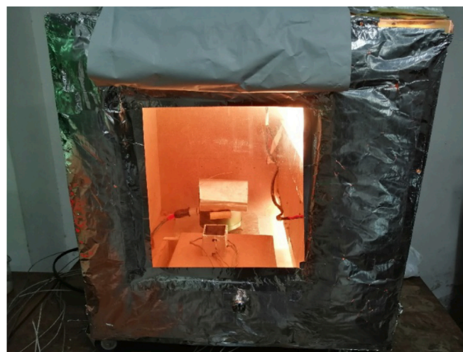
Fig. 1. Testing Chamber with glass wool and Aluminum foil insulation.
