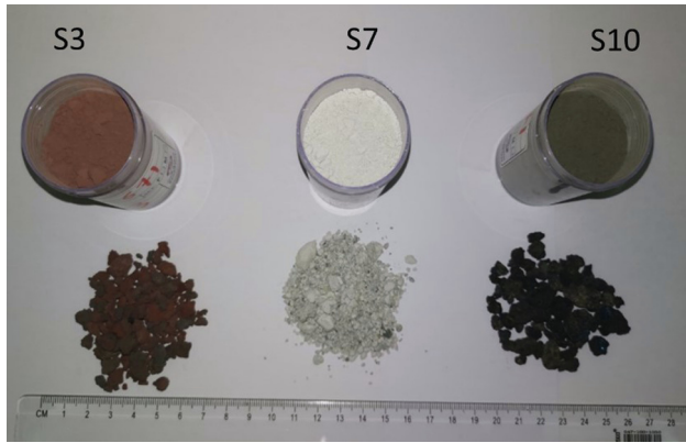
Fig. 1. Raw (on the bottom) and powder (on the top) volcanic ash of the selected samples S3 (poor red color), S7 (white color), and S10 (black color).
