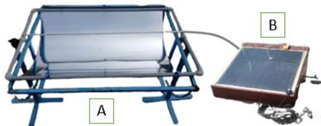
Fig. 1. (A) shows a photograph of a linear compact parabolic trough collector with receiver. Fig (A) and (B) Parabolic trough Integrated solar still.
