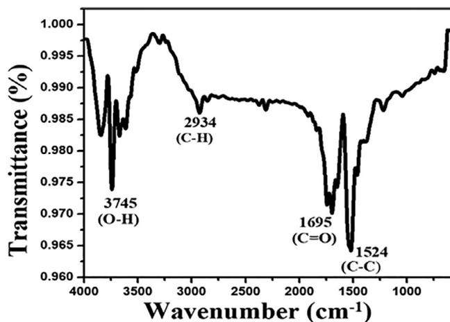
Fig. 3. FTIR spectra of *B. laciniosa* mediated AuNPs.
