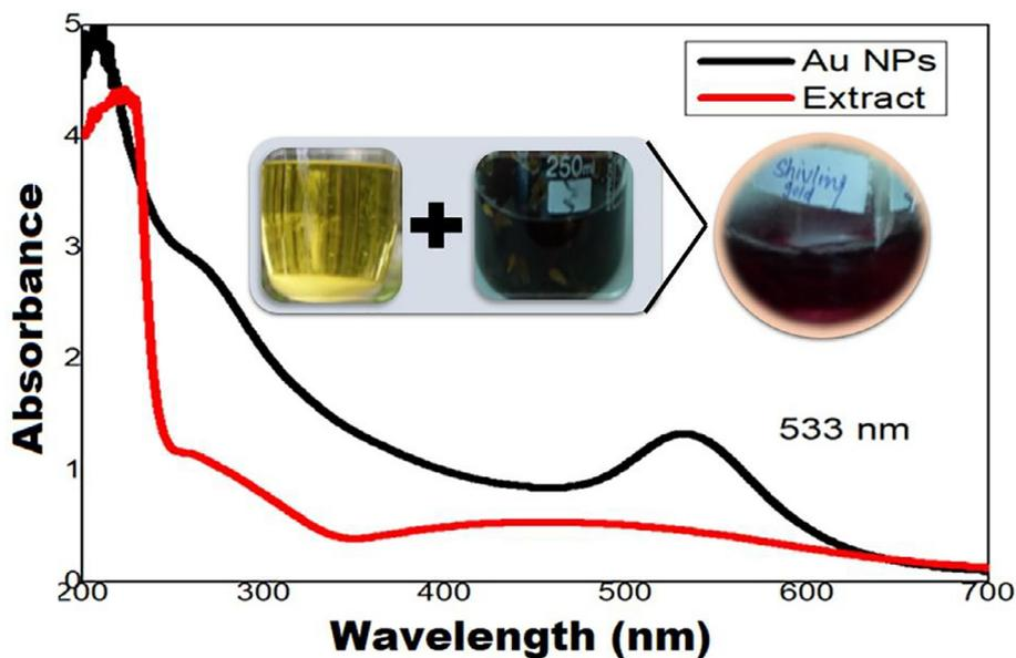
Fig. 2. UV-visible spectra of synthesized AuNPs and *B. laciniosa* seed extract.
