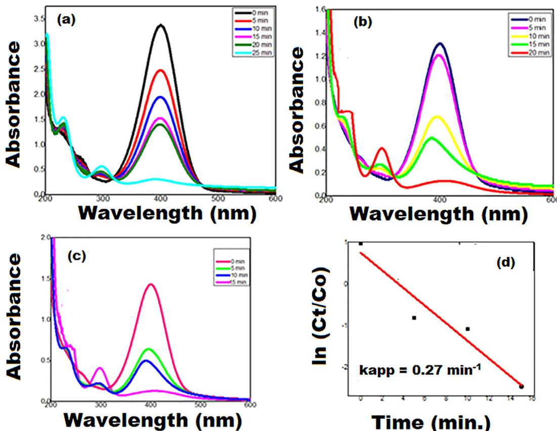
Fig. 6. (a–c) Catalytic efficacy of 4-NP in various concentrations (5, 10, and 15  $\mu\text{L}$ ) and (d) kinetic studies.
