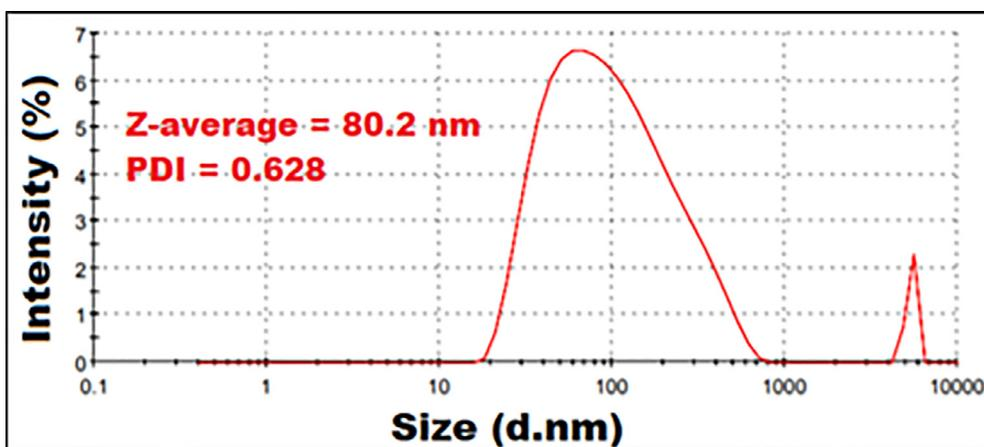
Fig. 5. Zetasize analysis of *B. lacinososa* mediated biogenic Au NPs.
