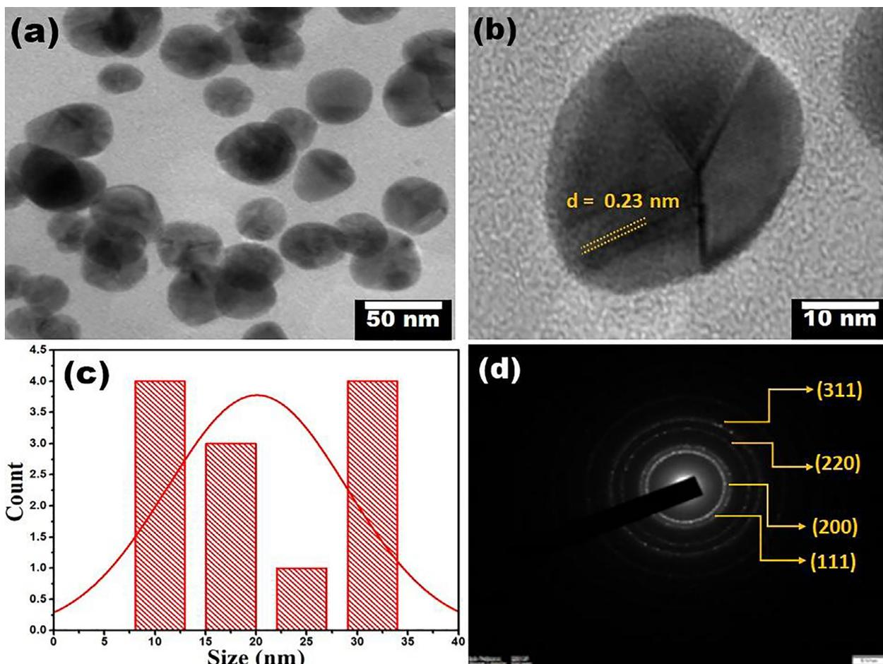
Fig. 4. Microscopic analysis of Au NPs: (a-b) HR-TEM micrographs with lattice d-spacing, (c) histogram with size distribution curve, and (d) SAED pattern with corresponding crystal planes.
