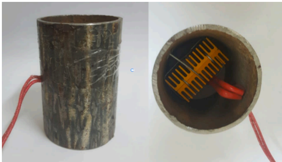
Fig. 2. A battery model made instead of a real battery.
