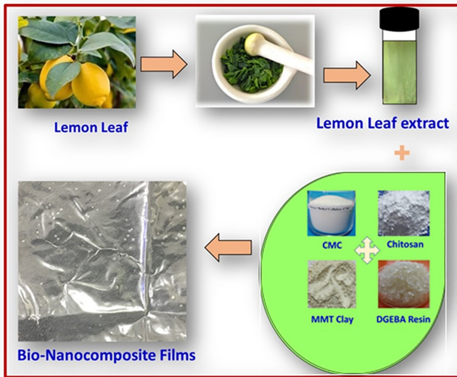
Fig. 1. Schematic representation of the bio nanocomposite films prepared adding the lemon leaf extracts.
