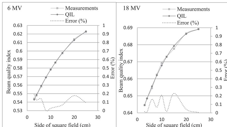
Fig. 4. Beam quality index law (QIL) and committed error variation as a function of field size.
