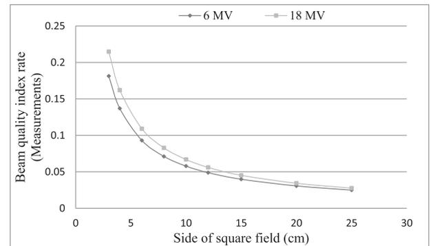
Fig. 5. Beam quality index rate variation as a function of field size.
