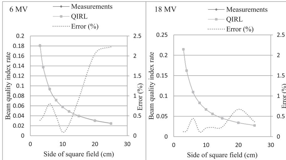
Fig. 6. Beam quality index rate law (QIRL) and committed error variation as a function of field size.
