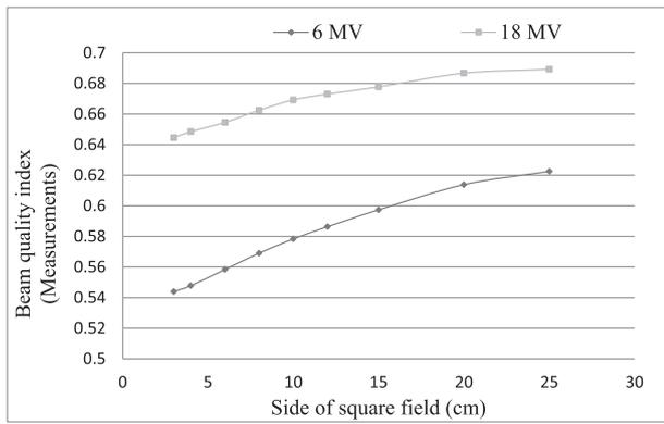
Fig. 3. Beam quality index variation as a function of field size.
