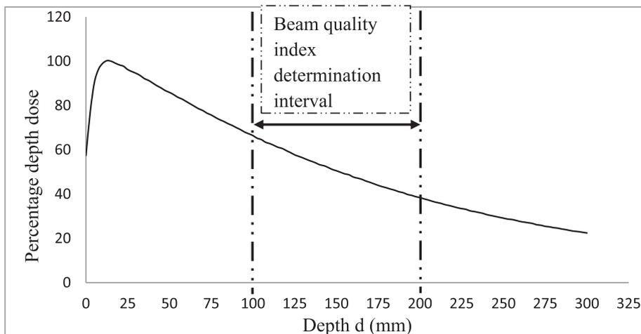
Fig. 1. Percentage depth dose variation as a function of depth and depths interval of beam quality index determination.
