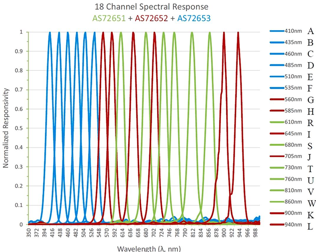
Fig. 2. 18 channel spectral response of AS7265X sensors (Alshami et al., 2024).
