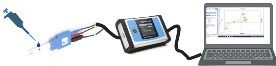
Fig. 1. Experimental setup used for the detection of DENV antigen using the immobilized carbon chips connected to potentiostat and measuring the change in potential using LSV by the software PSTrace 5.8.
